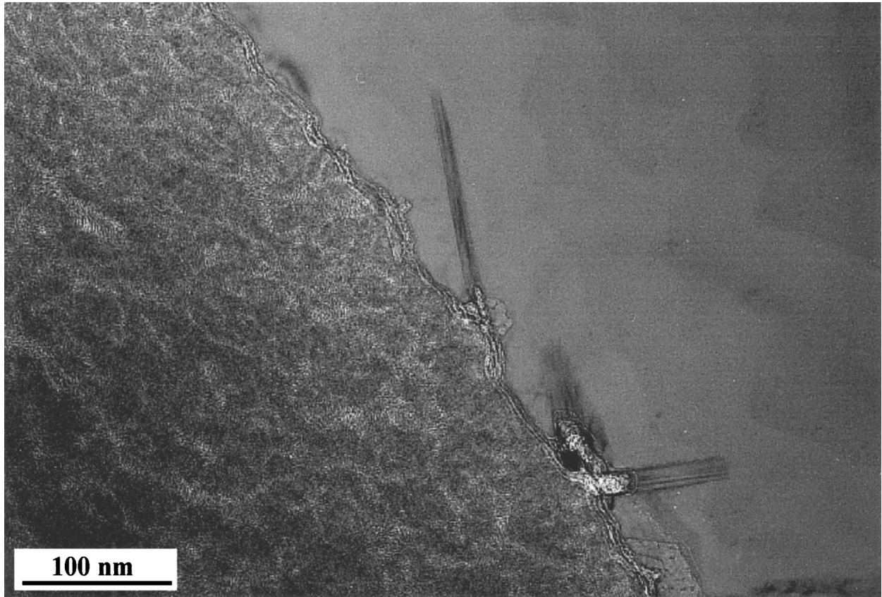
Figure 10 Carbide needles located at graphitic agglomerations.
