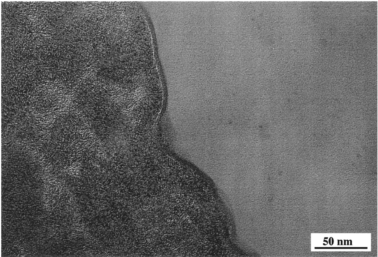
Figure 8 Nanometre-sized interlayer between fibre (left) and matrix (right).
